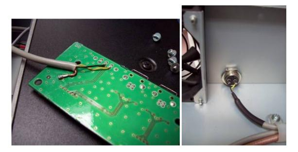
While the RP-4000 was opened up the opportunity was taken to replace the internal RG-58 coax cables originally fitted by ICOM.
