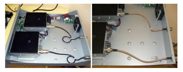
The following are pictures of the completed modified RP-4000 and the MT Climie D-Star rack installation.
