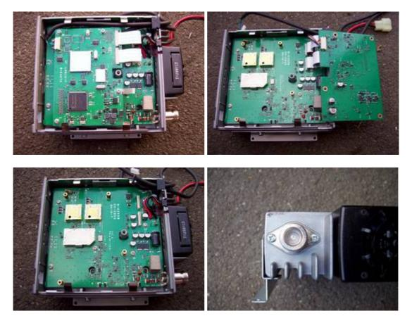
The power block heat sink surface is not milled flat and has a rough surface. Excess heat grease was used and has melted and pooled into hard lumps.
