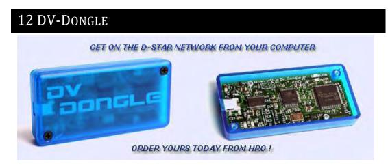
The DV Dongle costs about \$299. It is essentially an AMBE chip plugged on a card that allows a user to connect to any DPlus enabled gateway. In short if the repeater has a gateway with DPlus on it, you can connect to it.
