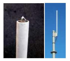
With a high speed cutting disk the resin knob was cut off. The tuning stub could now be adjusted. A sliver plated 3mm diameter wire was used to fine tune the antenna. After tuning a new cap is resin filled and placed back on top. A small 2mm hole is required to release the air as it is pushed on. Tape around the hole until the resin has hardened.
